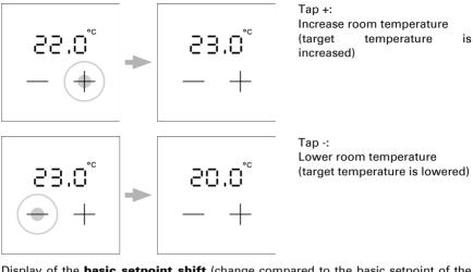
Display of the **basic setpoint shift** (change compared to the basic setpoint of the control):
