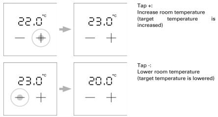
Display of the **basic setpoint shift** (change compared to the basic setpoint of the control):
