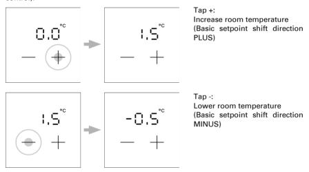
Option C: Display of actual temperature and target temperature/basic setpoint shift
