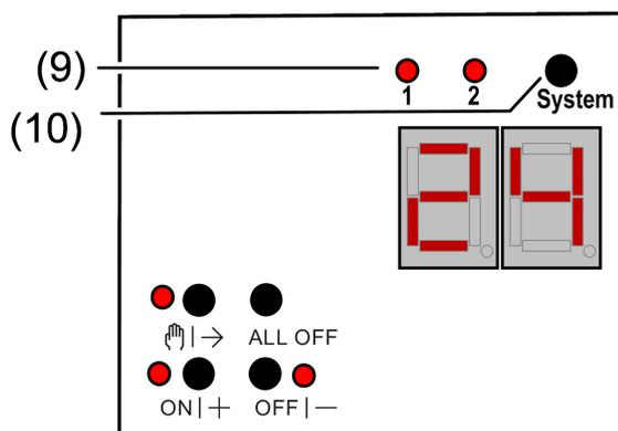
Figura 2: Panel de control DALI Gateway doble
