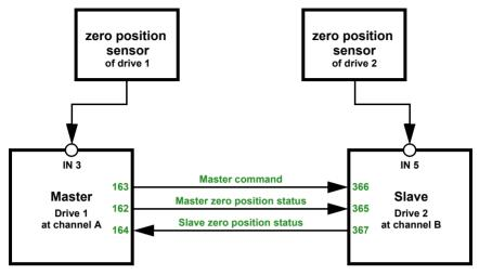
Drive channel A is Master, zero position sensor at input 3 of the actuator, drive channel B is Slave, zero position sensor via bus:
