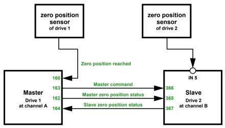
Drive channel A is Master, zero position sensor via bus, drive channel B is Slave, zero position sensor via bus:
