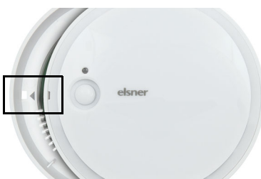
Fig. 7 Close the housing by positioning the cover and snapping it into place. To do this, align the recess on the cover to the marking on the skirting (the presence sensor must protrude through the opening in the cover).
