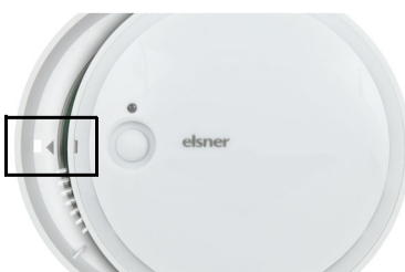
Fig. 7 Close the housing by positioning the cover and snapping it into place. To do this, align the recess on the cover to the marking on the skirting (the presence sensor must protrude through the opening in the cover).
