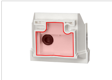
Fig. 6 a+b a) If the power lead is to be hidden when installed, it must emerge from the wall in the vicinity of the rear of the housing (marked area).
