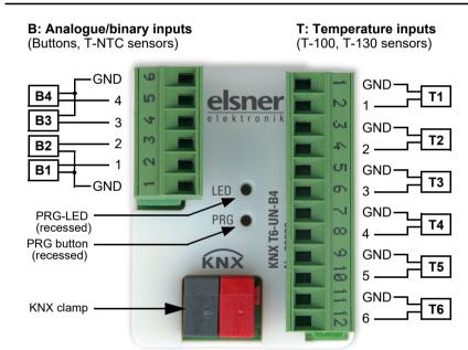
The cables of the T-100, T-130 and T-NTC temperature sensors can be extended to a maximum of 10 m.
