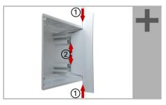
Adjust the screws of the magnetic mounting with the enclosed template. Each of the four screws must be adjusted individially in height.
