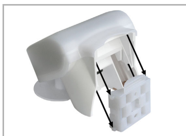
Fig. 15 Push the housing from above into the fastened mount. The bumps on the mount must snap into the rails in the housing.
