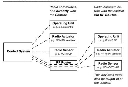
Radio actuators (ventilators, relays, motor control units ...) can only be operated with the remote control Remo 8 *via the control*. They can *not be additionally* switched directly with the remote control.
