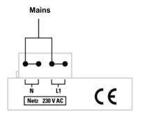
The **RF-Router-UP** only needs a mains connection.
