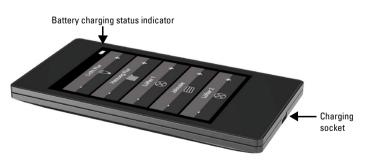
First, charge the integrated battery of the remote control with a standard commercial USB charging device (USB 2.0 Micro B connector). Charging will reset the transport block that is active on delivery. The remote control can be used only once it is connected to the power supply via the charger.
