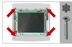
Screw the adapter plate with the WS1 Color onto the WS20 concealed box.
