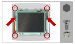
Screw the WS1 Color display unit onto the adapter plate with the screws provided. The nuts must show to the rear.
