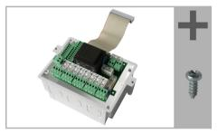
Remove the WS1 Color circuit board from the concealed box and mount it in the WS20 concealed box.
