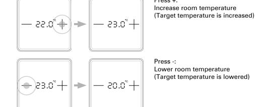
Display of the basic setpoint shift (change compared to the basic setpoint of the
