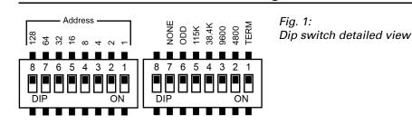
If all the dip switches are in the OFF position (factory settings), the following parameters are set:
