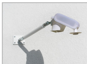
Fig. 6 Different mounting arms are available from Elsner Elektronik as additional, optional accessories for flexible installation of the weather station on a wall, pole or beam. Example of the use of a mounting arm: Due to flexible ball joints, the sensor can be brought into ideal position.
