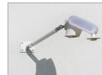
Fig. 7 Different mounting arms are available from Elsner Elektronik as additional, optional accessories for flexible installation of the weather station on a wall, pole or beam (pictures of sensors exemplary). Example of the use of a mounting arm: Due to flexible ball joints, the sensor can be brought into ideal position.
