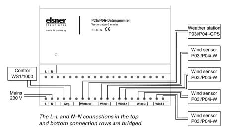
The connection is made with off-the-shelf UV-resistant telephone cable (A-2Y(L)2Y 2x2x0.6 or A-2Y(L)2Y 2x2x0.8). The weather station, wind sensors and control can be connected with polarity disregarded.
