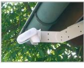
The hinge arm mounting extends the weather station from under the roof eaves. Sun, wind and precipitation can thus freely act upon the sensors.
