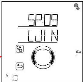
SP 09 (wind alarm)
