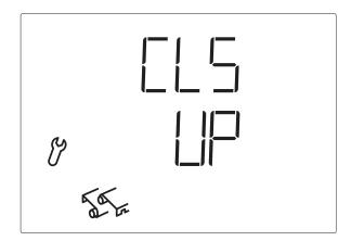
If the up and down connection cables have been mixed up when connecting the drive mechanism, this may be corrected in this step. First open the window a little bit for the rotational direction test. Check both arrow keys and make a setting in the display, whether the window closes again with  $\nabla$  or with  $\triangle$ .
