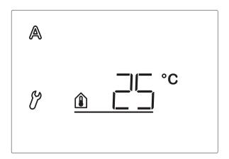
As soon as the value indicated here is exceeded, the automatic opens the window (unless the blocking value for the outdoor temperature has fallen below, see next parameter). The hysteresis is 2°C. That means, that the window will be closed as soon as the indoor temperature drops 2°C below the set value.
