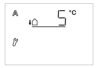
The outdoor temperature block keeps the window closed as long as the temperature is below the selected value. This means that in automatic mode, an opened window is closed and not opened again if the indoor temperature value (chapter A) is exceeded. Thus avoids energy losses during ventilation and protects plants from cold external air.
