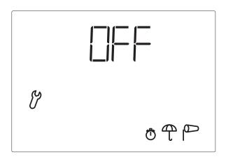
After the wind or rain alarm has been activated, the window is closed. The operating command for the connected drive mechanism either ends after 4 minutes or is permanently maintained as long as the alarm message exists. The permanent operating command is necessary if Arexa is used as control centre for wired motor drive units (e. g. IMSG 230) which control several drive mechanisms.
