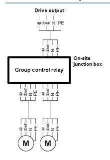
Drive group with a **total output of less than 500 VA** at the drive output of the weather station or at a motor control unit.
