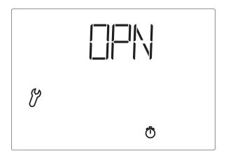
Now open the window as far as the automatic shall do it later. Then press the SET key in order to access the next setting step.
