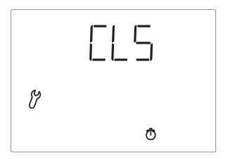
At first, completely close the window. Then press the SET key in order to access the next setting step.
