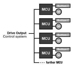
**Central control with group formation** with motor control units (MCU) at the drive output of Arexa weather station:
