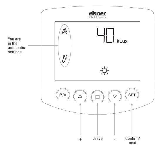
You may leave the automatic settings at any time by pressing the key  $\Box$ . The accomplished changes of the values are not saved in this case.
