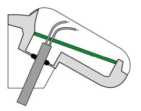
Remove the cable shielding under the circuit board and only feed the connector cables upwards through the openings in the circuit board.
