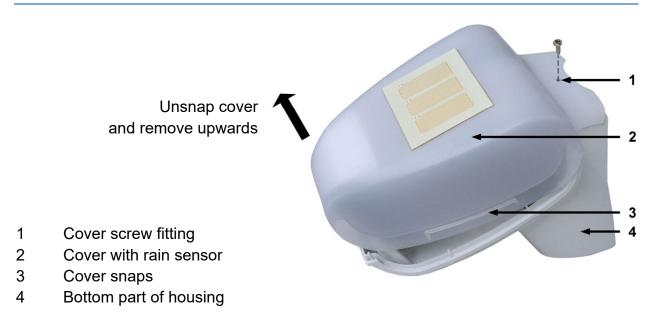
The cover of the weather station with rain sensor is engaged at the lower rim to the right and to the left (see fig.) Remove the cover from the weather station. Be careful not to break away the cable connection between the circuit board in the bottom part and the rain sensor in the cover.
