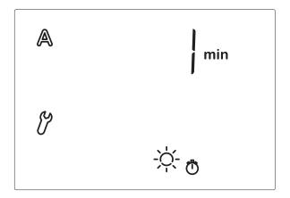
The purpose of the delay is that the shading does not permanently extend and retract in case of fast changing lightness conditions.
