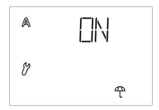
The rain alarm protects the exterior shadings, particularly awning fabric, from damage. In case of rain alarm, the shading is automatically retracted and manual operation is blocked.
