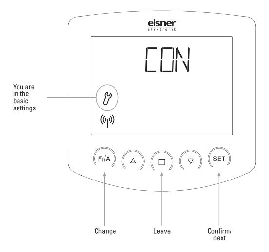
You may leave the basic settings at any time by pressing the key  $\Box$ . The accomplished changes are not saved in this case.
