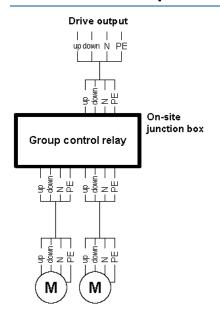
Drive group with a **total output of less than 500 VA** at the drive output of the weather station or at a motor control unit.
