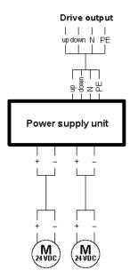
Drive group with **DC motors** at the drive output of the weather station or at a motor control unit.
