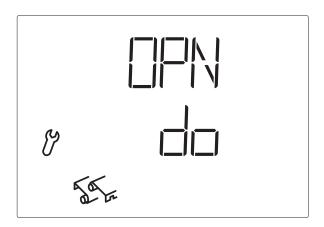
If the up and down connection cables have been mixed up when connecting the drive mechanism, this may be corrected in this step. First extend the shading a little bit for the rotational direction test. Check both arrow keys and make a setting in the display, whether the shading retracts (i.e. opens) with  $\nabla$  or with  $\triangle$ .
