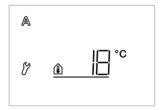
By means of the indoor temperature block, you may use the sun in order to obtain the desired room temperature (e.g. in winter). Only if the value is exceeded, the shading extends in case of sun. The indoor temperature is only applied for the automatic mode of the control system. The manual operation of the shading is still possible.
