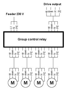
Drive group with a **total output of more than 500 VA** at the drive output of the weather station or at a motor control unit. The possible total output depends on the group control relay.
