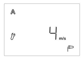
The wind alarm protects the exterior shadings from damage. If the indicated wind value is exceeded, the awning or blind is retracted and manual operation is blocked.
