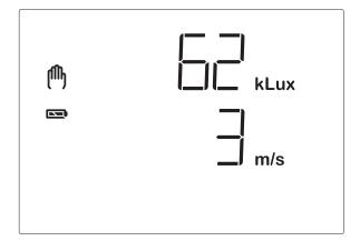
Note: During the first approx. 90 seconds after the return of voltage at the weather station, the wind value is not displayed correctly (e.g. after a power fail or in case of a first start). Therefore, manual operation is blocked in this period of time in case of activated wind alarm.
