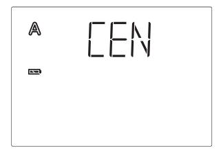
In order to get to the display, press key  $^{\bigcirc}/^{\triangle}$  twice shortly in automatic mode ( $^{\bigcirc}$ ) and once shortly in manual mode ( $^{\bigcirc}$ ).
