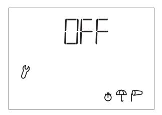
After the wind or rain alarm has been activated, the shading is retracted. The operating command for the connected drive mechanism either ends after 4 minutes or is permanently maintained as long as the alarm message exists.
