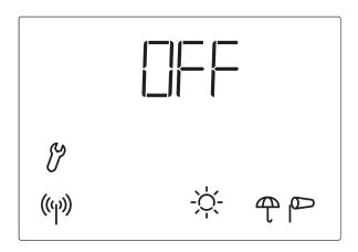
Leave this display at TFF if Solexa is used as conventional single-channel control system. The function "Sending of weather and automatic data" must only be activated if Solexa shall cooperate with motor control devices (e.g. XS MSG2-AP) in the control system XS.
