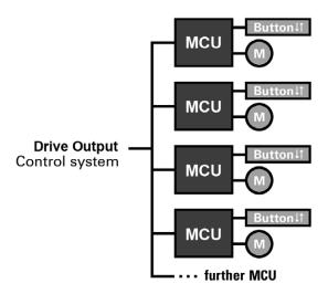
**Central control with group formation** with motor control units (MCU) at the drive output of Solexa weather station:
