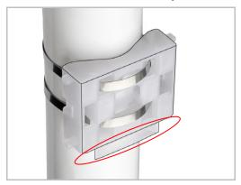
When pole mounting: curved side on pole, collar downward.
