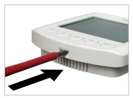
Open the operating unit by unlocking the locking at the lower rim of the housing. For this purpose, you must press with a screwdriver straight into the gap.
