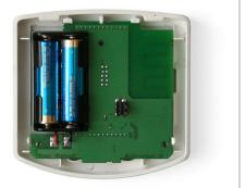
Observe the correct polarity of the batteries. You need two standard batteries (1.5 V) or accumulators (1.2 V) of type AA (Mignon/ LR6).
