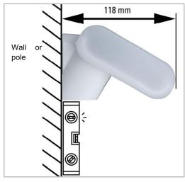
The weather station must be mounted on a perpendicular wall (or a pole).
