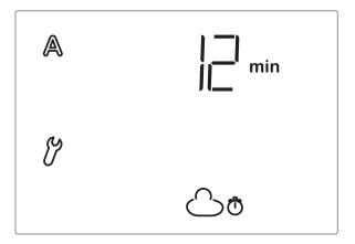
The presetting for the retraction is 12 minutes. Thus, for 12 minutes, the lightness must be continuously lower than the value which you have set (topic A of the automatic settings) for the extended shading to retract. Thus, clouds passing by are "ignored".
