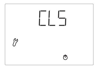
Now extend the shading as far as the automatic must extend it later in case of sunshine. Press the SET key in order to access the next setting step.
