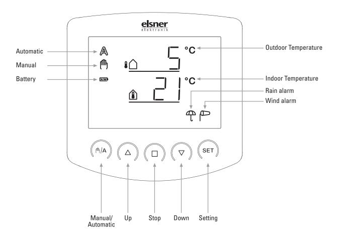
The basic position of the operating unit of the control system displays the current outdoor temperature (upper line) and the indoor temperature (lower line) as well as the function mode (automatic or manual), the battery load and the current alarm messages for rain or wind. The meteorological data are updated once per minute (and in case of a keystroke).
