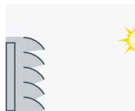
The slats of the blind are adjusted according to the height of the sun
