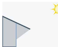
The sun automation takes into account the shadow cast by the roof overhang and knows the shadow edge
