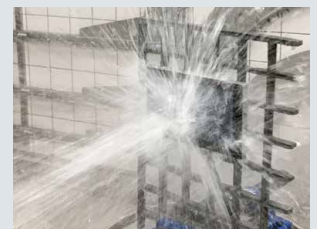
Jet water test
